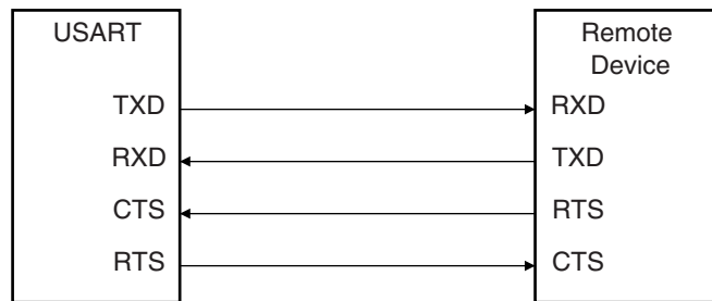
Figure 31-19. Connection with a Remote Device for Hardware Handshaking
